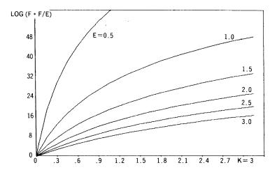
Fig. 1 (a) Relative value of the coincidence probability F of two deuterons interacting with a screened Coulomb potential is plotted as a function of the screening constant  $\kappa$  with a parameter E (mutual energy). The standard is taken at  $\kappa=0$ . The WKB approximation is used in the calculation.
