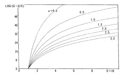
Fig. 2 (a) Relative value of the coincidence probability of two deuterons interacting with a screened Coulomb potential G is plotted as a function of the mutual energy E with a paramethr  $\kappa$ . The standard is taken at E=1 (in a. u.).
