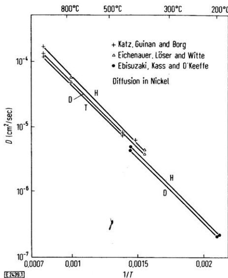
Fig. 3.1 Diffusion coefficients of hydrogen, deuterium and tritium in nickel [Birnbaum 1972]
