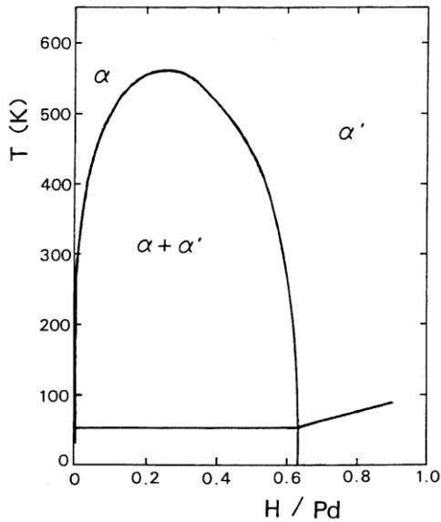
Fig. 1.8 Phase diagram of the Pd-H system which is very similar to that of the Pd-D system [Fukai 2005]
