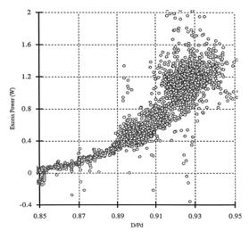
Fig. 5. Variation of excess power with loading ratio D/Pd obtained by McKubre et al. [9].
