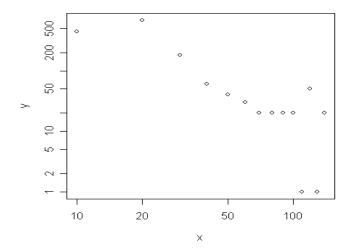
Fig. 4. Distribution of the frequency  $N_P$  (= y) producing excess power  $P_{\rm ex}$  (= x). To depict log-log curve, values of  $N_P$  and  $P_{\rm ex}$  were arbitrarily multiplied by  $10^{\rm n}$ . (x = 100 in this figure corresponds to  $P_{\rm ex} = 1$  W)
