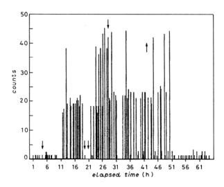
Fig. 7. Diagram showing the time evolution of the neutron emission counts (ordinate) during the first run (7-10 April, 1989) by De Ninno et al. [16]. The values indicated are integral counts over periods of 10 minutes.
