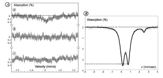
**Figure 1.** *A*, Mossbauer spectra of Fe<sup>57</sup> isotope of *Saccharomyces cerevisiae* culture grown in nutrient medium in the presence of (*a*)  $D_2O$  and  $Mn^{55}$ ; (*b*)  $H_2O$  and  $Mn^{55}$  and (*c*)  $D_2O$  without  $Mn^{55}$ . *B*, Mossbauer spectrum of MCT grown in nutrient medium in the presence of  $D_2O$  and  $Mn^{55}$  isotope.
