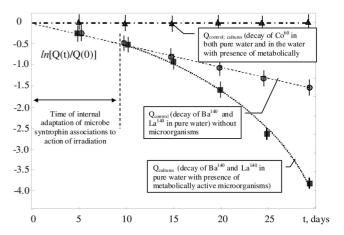
**Figure 3.** Activity Q(t) of the same reactor Ba<sup>140</sup>, La<sup>140</sup> and Co<sup>60</sup> isotopes in the experiment on transmutation (activity  $Q_{\text{cultures}}$  in pure reactor water in the presence of MCT) and in the control (activity  $Q_{\text{control}}$  in the same water without MCT).
