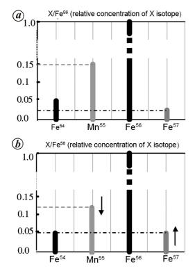
Figure 2. Mass spectrum of iron region of microbiological associations (dried biological substances) that were grown in control nutrient medium with  $H_2O$  and  $Mn^{55}$  (*a*) and in experimental nutrient medium with  $D_2O$  and the same amount of  $Mn^{55}$  isotope (*b*).
